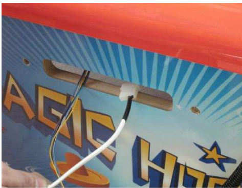
15. Lamp connection for models; MAGIC, GAMELAND Plug in a lamp's cable (12V) with cables of a cabinet.
